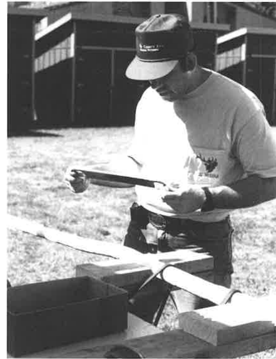
▲ Larry is using a manually operated pole peeler to make log furniture.
